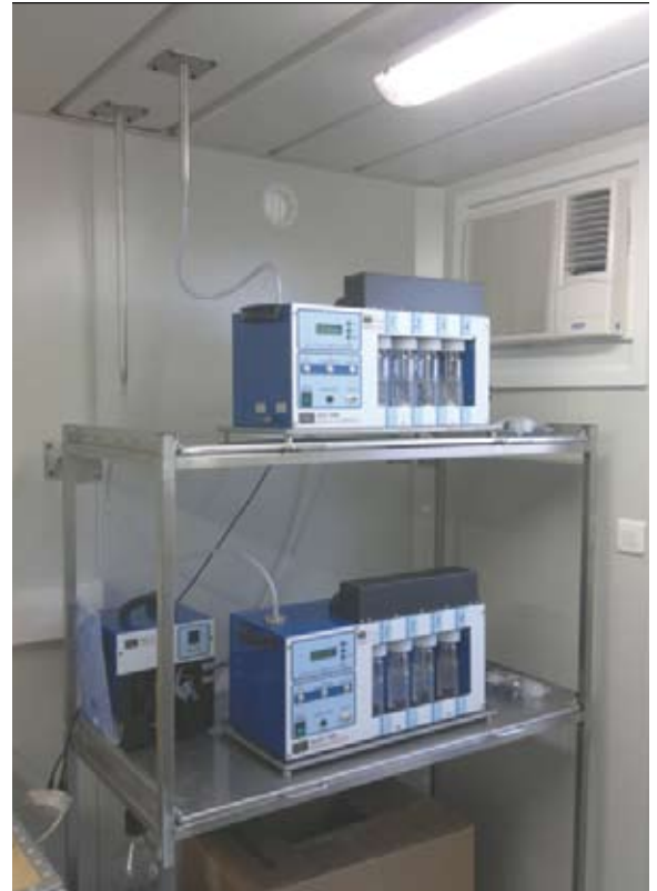
MARC 7000 tritium and HAGUE 7000 carbene 14 samplers installed on a stainless steel shelf, with atmospheric sampling probes.
