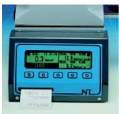
The NT200 calibration is done very easily with an automated procedure. The activity of the reference source, the measuring time and the step high voltage for the plates must be selected. The NT200 automatically selects the start and stop high voltage and computes the detector response curve which is displayed in real time on the screen.
