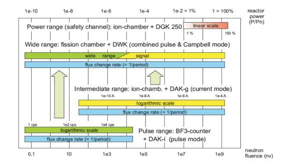
Measuring ranges of the neutron flux instrumentation. Example for the PWR
