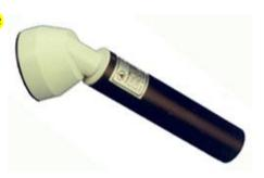
A low voltage interface connects the <u>RAM DA 2000</u> monitor with the probe. The GM-10 uses a pancake GM detector with a thin mica window. This is encased in a rugged, splash proof housing for protection against shock, vibration and humidity. The probe also contains a high voltage power supply, pulse shaper, GM saturation indicator, detector identifier and malfunction detection circuitry. This configuration minimizes noise, improving sensitivity and stability.
