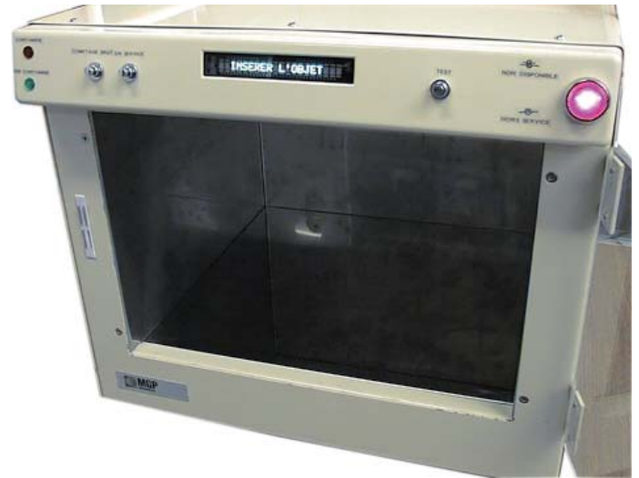
The measurement chamber is made out of polished stainless steel permitting easy decontamination
