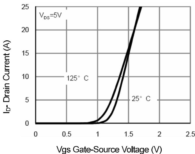
**Figure 7 Transfer Characteristics**
