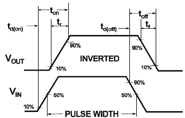
**Figure 2:Switching Waveforms**
