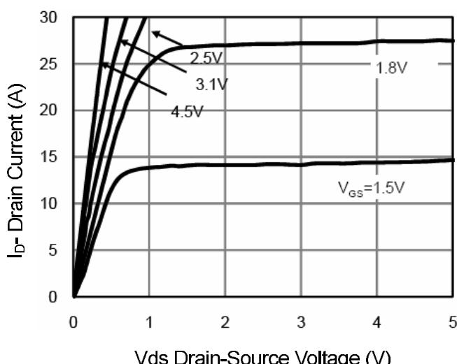
**Figure 5 Output Characteristics**
