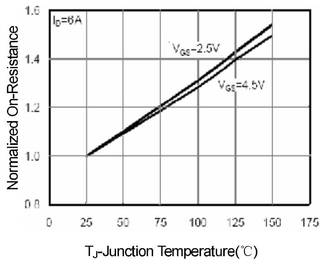
**Figure 8 Drain-Source On-Resistance**
