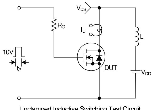
Undamped Inductive Switching Test Circuit
