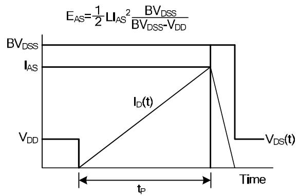
Undamped Inductive Switching Waveforms
